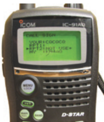
Figure 4 — Part of the extensive menu system on the IC-91AD handheld. It takes a minute to get used to what YOUR call sign and MY call sign mean. To talk to anyone, you program CQCQCQ in the YOUR field. If you wanted to talk to a specific station, you'd program that station's call sign in the YOUR field. If you want to use specific linked repeaters, you use the RPT1 and RPT2 fields. This is one radio you can't operate without some quality time in the manual.
